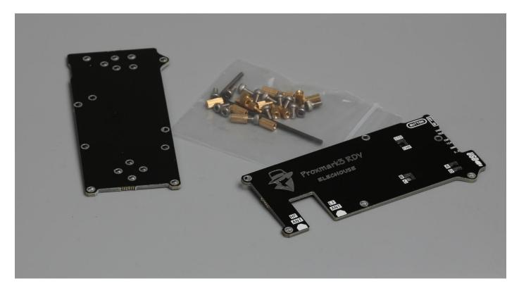
This protector is made of RF4, which is the same material as the main board. This protector mainly prevent the Proxmark main board from being touched during working. Touching the board might cause interference to it while it is working.
